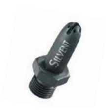
**SILVENT 811:** "PEEK" nozzle with a central orifice. Withstands aggressive chemical environments, corrosive cutting fluids and temperatures of up to 260°C (500°F). Protects sensitive products against scratching and impact. 1/8" male connection thread.
